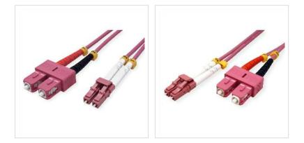
OM4 fiber for existing 1 and 10 Gbit/s applications as well as future 40 and 100 Gbit/s systems. Allows extended reach upwards of 550 meters at 10 Gbit/s for ultra long building backbones and medium length campus backbones. With an laser bandwidth of 4700 MHz-km (more than double the IEEE requirement for 10 Gbit/s 300 meter support), the OM4 fiber is also especially well suited for shorter reach in data centers and high performance computing applications.
